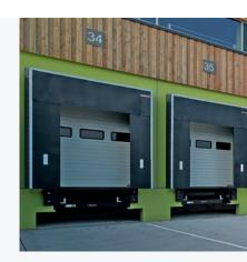
For temperature-controlled buildings, we provide thermal insulation solution by a thermal insulated sectional door positioned in front of the telescopic dock leveller, to minimize thermal losses during the periods that goods are not being loaded at the loading bay and the door is closed.
