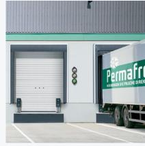
To fully utilized your space in the workshop, you can move the dock leveller into loading house in front of the building. The hydraulic dock leveller allows docking of lorries with different loading heights. In addition, the double-skinned insulated industrial door seals the building well.
