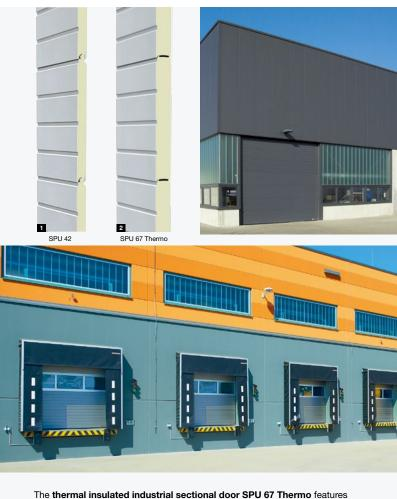
good thermal insulation with sections with thermal break, depth 67 mm, lowering temperature losses at door openings, making it ideal for use in food, cold logistics and commercial buildings. This also reduces the formation of condensation water inside of the door.
