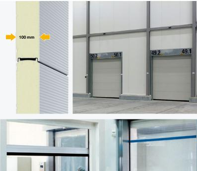
Thanks to its 100 mm sections with thermal break and special seals for the building structure and floor, the **ISO Speed Cold** is the ideal solution for all areas with high temperature differences. Used as a high-speed door in cold-storage areas or to save energy in production and distribution areas, the **ISO Speed Cold** remains impervious.
